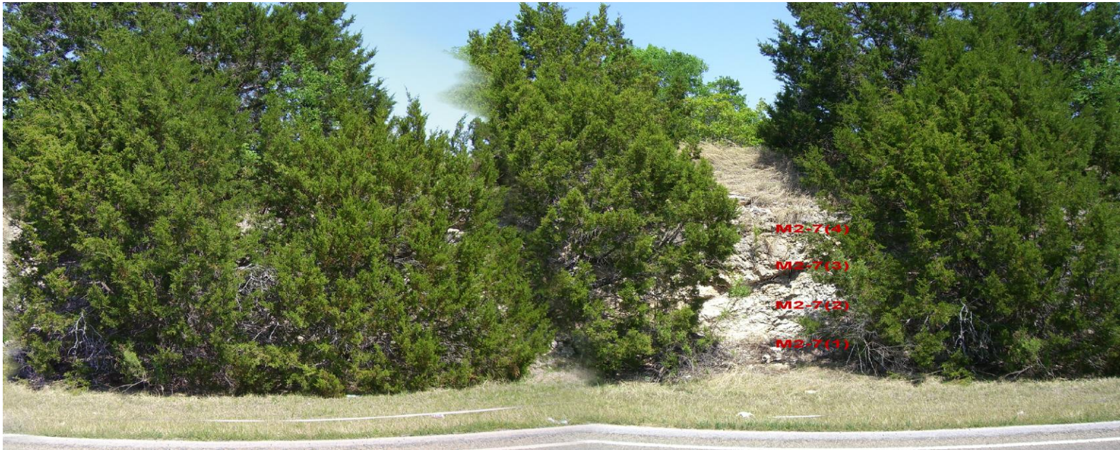
Figure A17. Composite panoramic 7 of 10: Mosheim-2 sampling locations. Column 7 is 26.5m from Column 6. Vertical sampling intervals were .6m.
