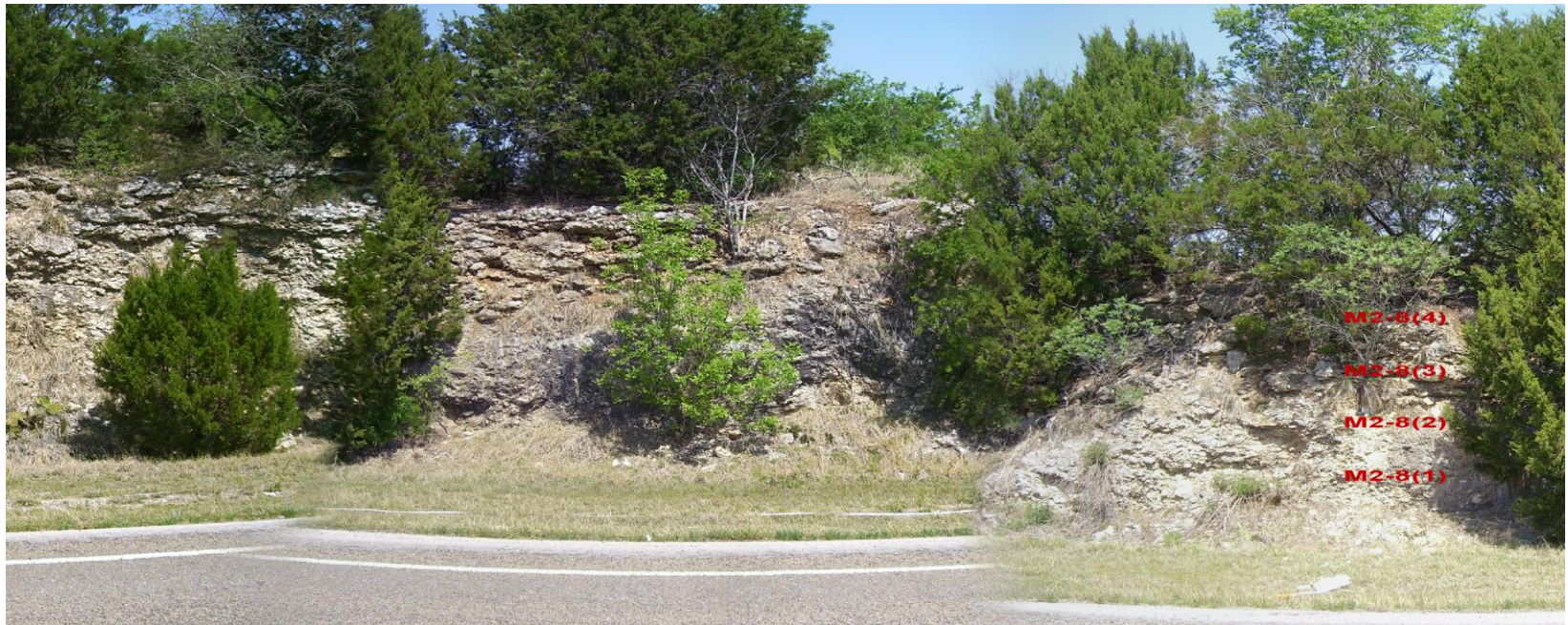
Figure A19. Composite panoramic 9 of 10: Mosheim-2 sampling locations. Column 8 is 24.4m from Column 7. Vertical sampling intervals were .6m.
