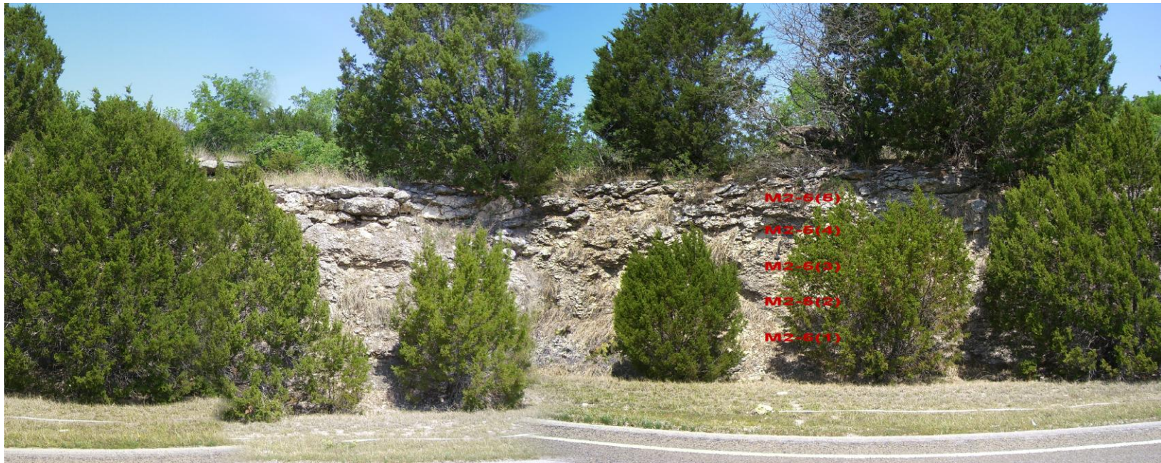
Figure A15. Composite panoramic 5 of 10: Mosheim-2 sampling locations. Column 5 is 32m from Column 4. Vertical sampling intervals were .6m.
