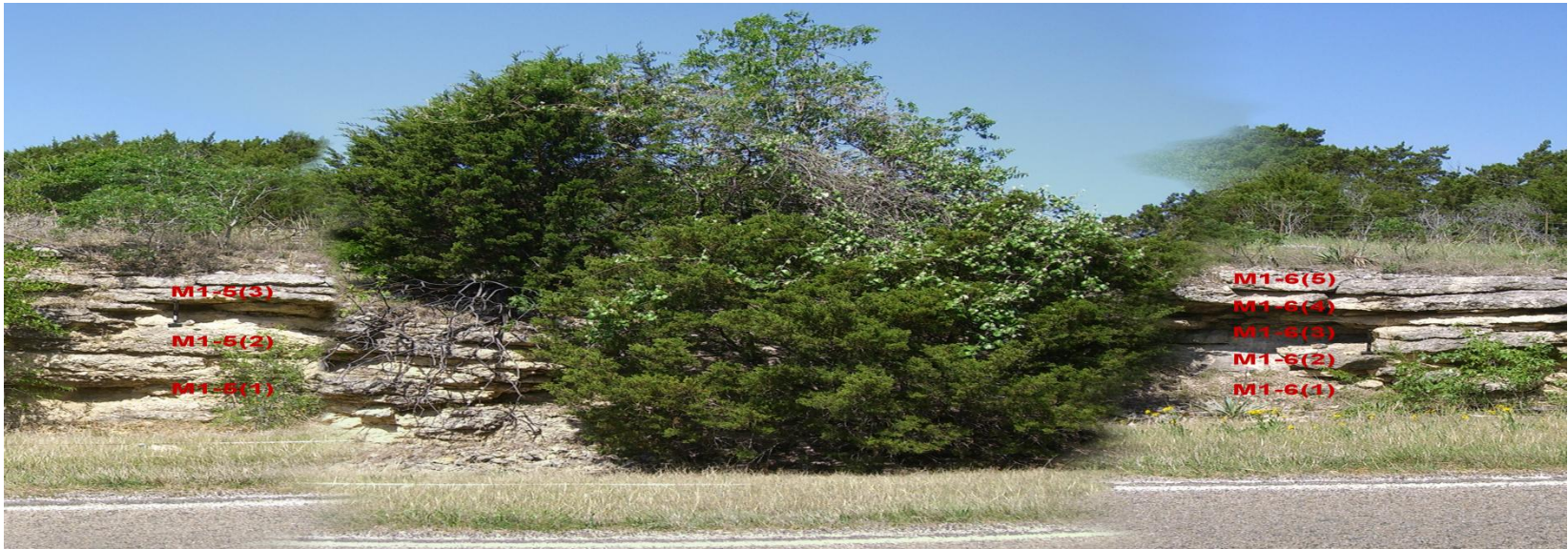
Figure A9. Composite panoramic 5 of 6: Mosheim-1 sampling locations. Column 5 is 10.8m from previous. Column 6 is 10.4m from column 5. Vertical sampling intervals were .6m for column 5 and 0.3m for column 6.
